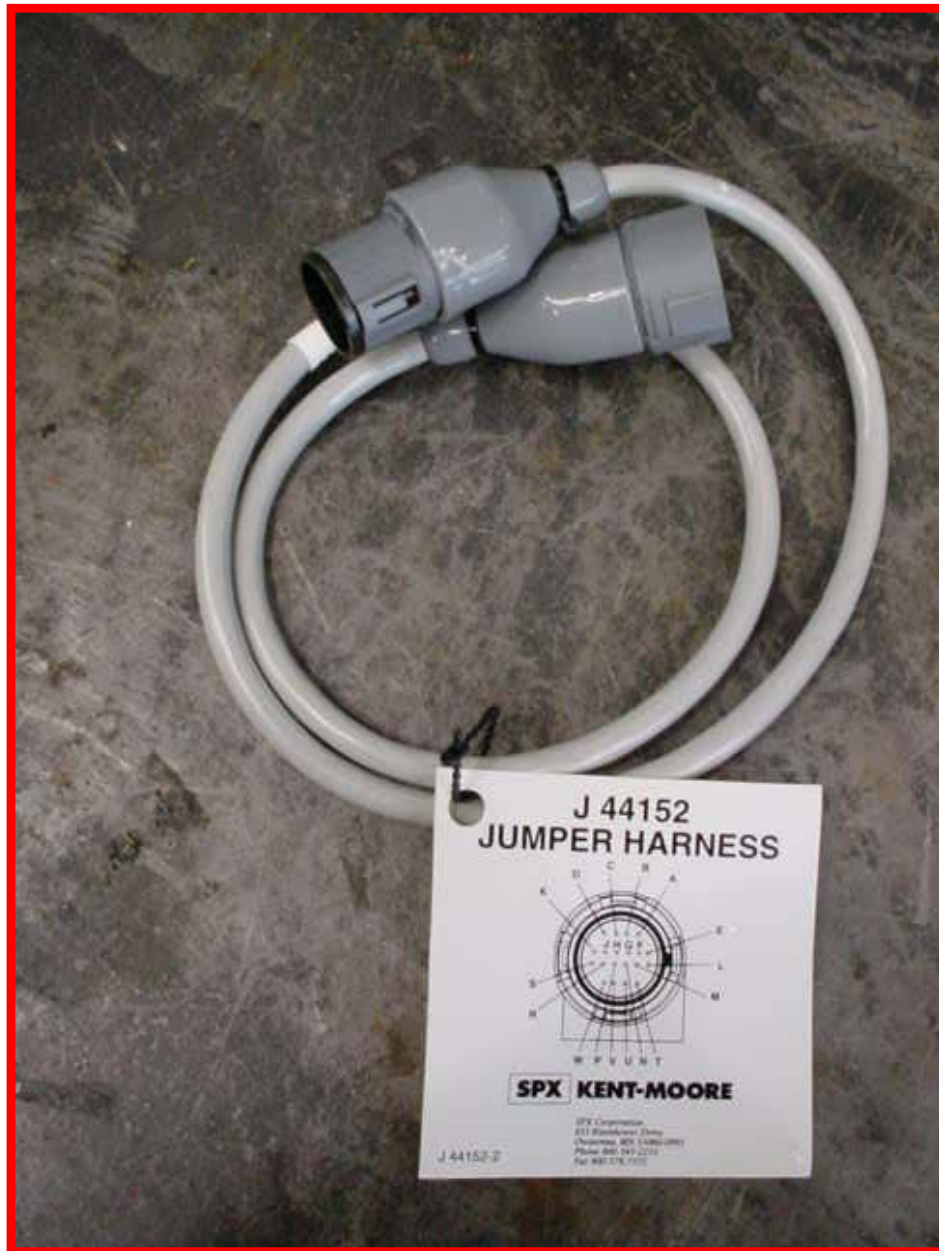
J 44152 Transmission Test harness (Kent Moore)
