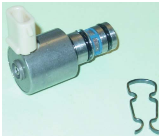
Figure 15. Torque Converter Clutch (TCC) PWM Solenoid.
