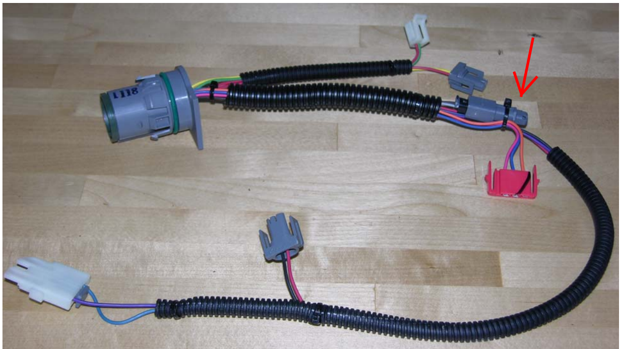
Figure 13. Transmission Fluid Temperature (TFT) Sensor
