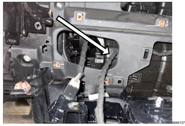
Note: The wire connector for the Trailer Brake Switch will be behind the Instrument Panel Accessory Bezel.
